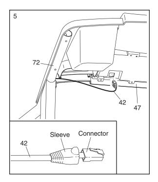
Set the Console Base (47) on the Handrails (71, 72).
